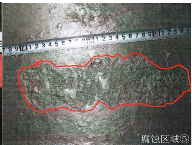
脱落处罐壁腐蚀减薄
